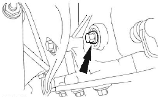
Fig. 347: Locating Engine Plug Bolt Courtesy of FORD MOTOR CO.
