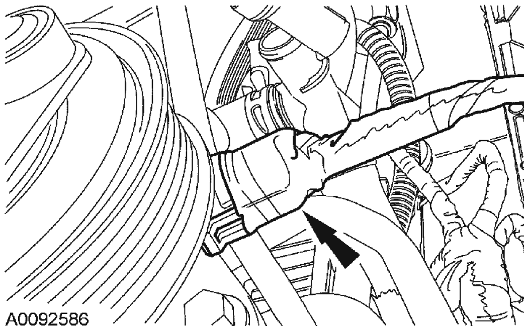
Fig. 264: Disconnect A/C Compressor Electrical Connector Courtesy of FORD MOTOR CO.
